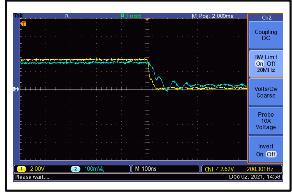
The Switching Fall Time is 200 ns
