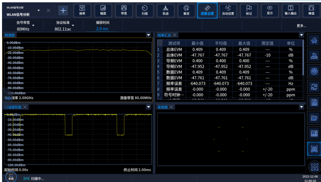
IEEE 802.11ac single user PPDU signal demodulation EVM 80MHz transmission bandwidth, QPSK+BPSK
