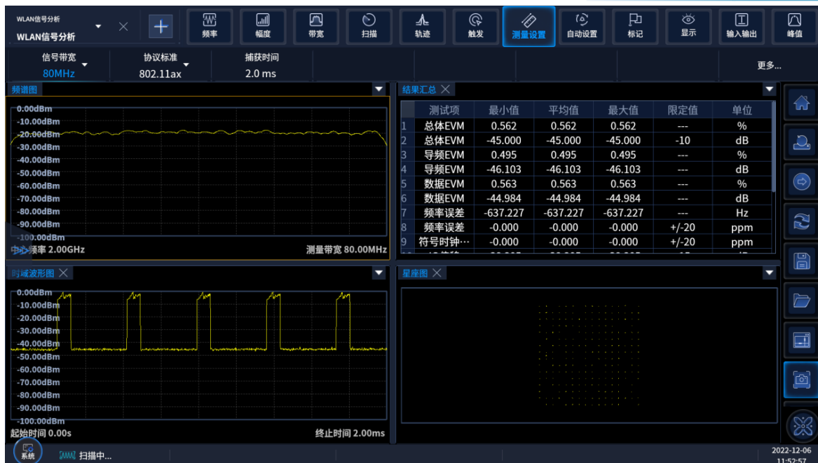
IEEE 802.11ax single user PPDU signal demodulation EVM 80MHz transmission bandwidth, 256QAM
