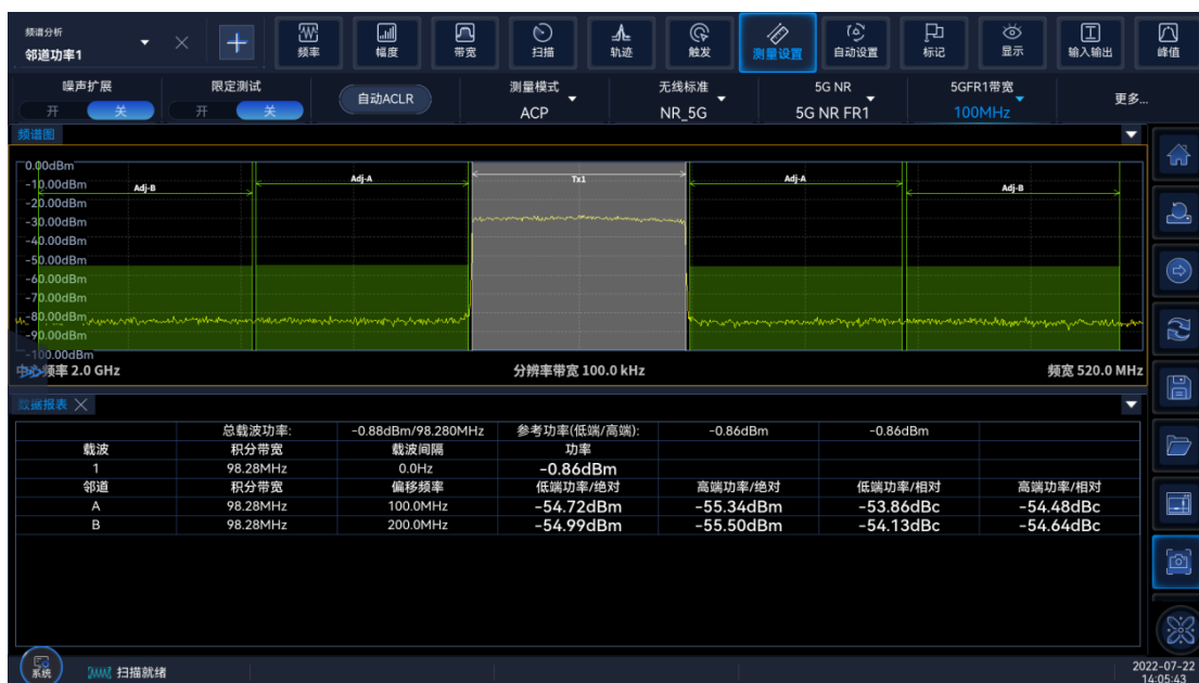
2GHz carrier 5G NR ACPR measured value
