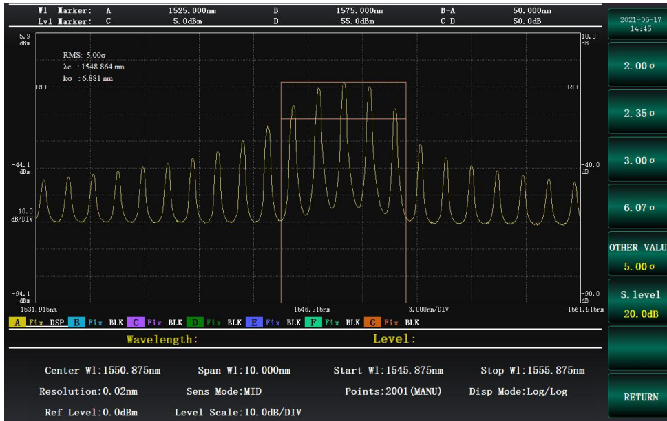
Center wavelength and bandwidth test based on root mean square analysis
