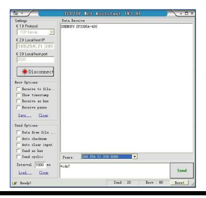
Note: the interface parameters must be identical to that of instrument settings, otherwise communication fails.
