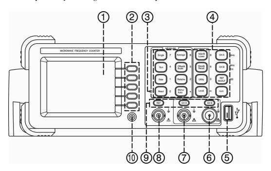
1 LCD display screen 5 USB Host 9 Indicator light of time base and channel
