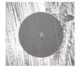
Contaminated (grease from hands) optical connector end-face
