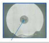
Photo showing a core that has melted as a result of a contaminated substance on the end-face being irradiated with a high power laser.
